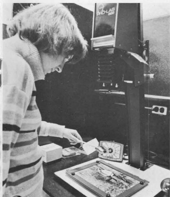
LEFT — Junior Sherry Marsh places holder with negative into the enlarger. With focus and timer set, Sherry exposes the print paper to the light; from there, the paper goes to the developer, from which it will leave as a final print.
